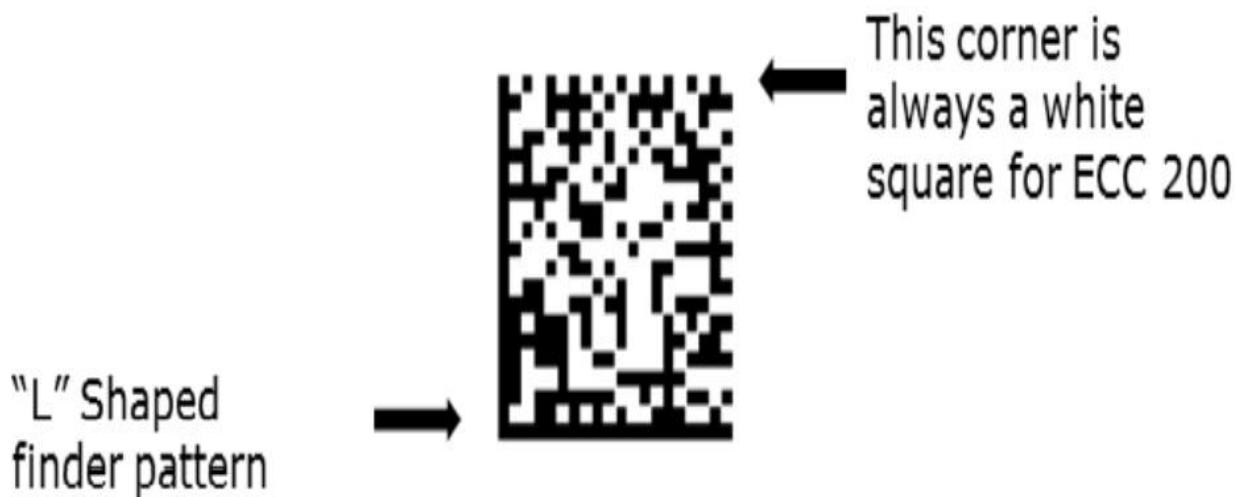
Figure 2: GS1 DataMatrix symbol adopted from GS1 General Specification
